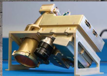
When delivered to the moon via CLPS, the Near-Infrared Volatiles Spectrometer System (NIRVSS) will detect the different types of minerals and ices present in the soil, including water.
